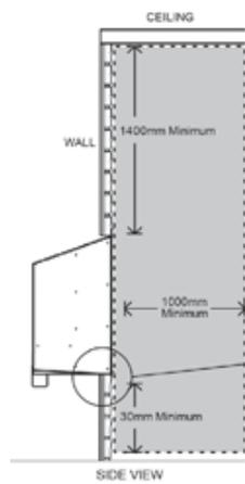
Minimum clearance distance between a combustible ceiling and the fascia must be no less than 1400mm.
