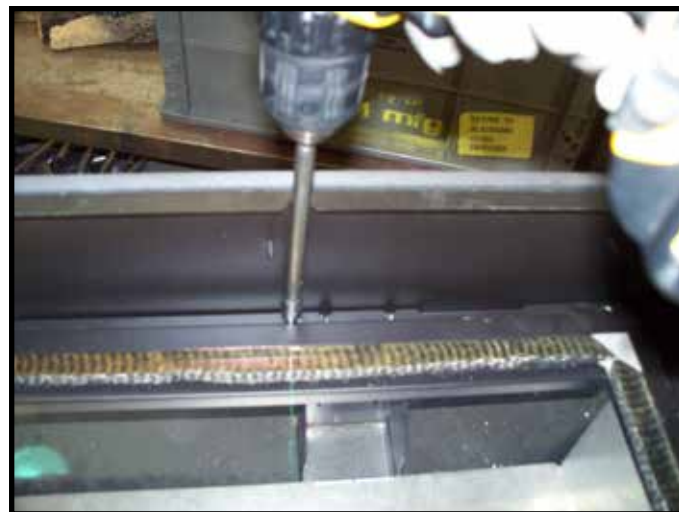
Figure 9.4. Gas and Electrical Access - Remove Glass Window
