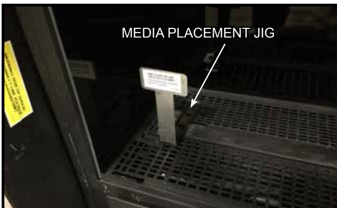
Figure 11.10 Media Placement Jig in Place
