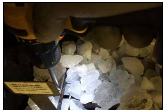
Figure 11.12 Remove Media Placement Jig
