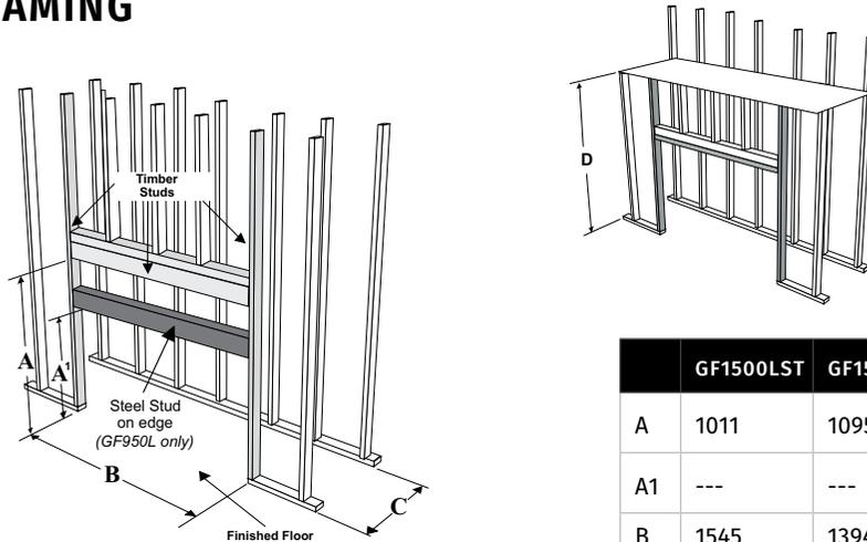
NOTE: Steel stud must be installed after unit has been positioned in place and prior to installation of non-combustible finishing
