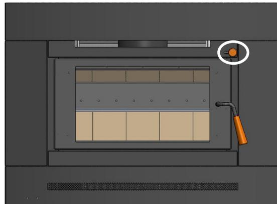
7. Install knob on damper control rod.
