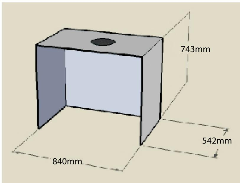
Ceiling requires 100mm airgap where flue penetrates (minimum 450mm diameter cutout).
