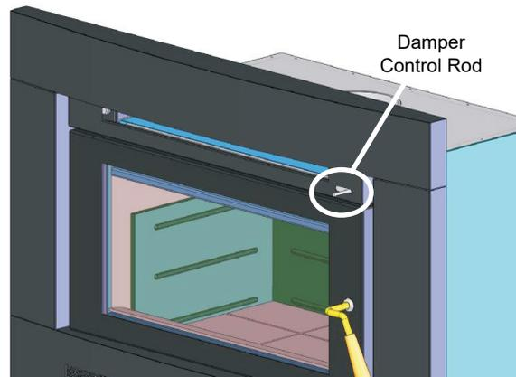
6. Install the draft plate cover by sliding the tabs into the tab brackets on the inside top of the firebox, ensure the damper control rod fits through the opening in the draft plate cover.
