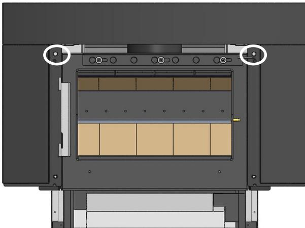
4. Install the fan fascia by aligning the bottom screw locations with the bottom faceplate. See page 13 for fan wiring diagram.
